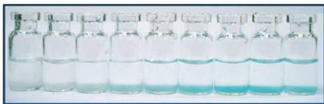
Fig. 8. Naked-eyes of F-oBOH-AMP/Gd 3+ CNPs@Cu 2+ in HEPES (0.1 M) pH 7.4 in the presence of different concentrations of CN - . From left to right ( \times 10 \mu\text{M} ): F-oBOH-AMP/Gd 3+ , 0, 2.0, 4.0, 7.0, 10.0, 20.0, 30.0, and 40.0.
